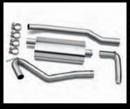
∼ CAT-BACK EXHAUST SYSTEM.<sup>(5)</sup> This system features T304 stainless steel construction with mandrel-bent tubing, stainless band clamps and polished tips. This free-flow system helps to provide horsepower and torque gains, improved fuel efficiency and a deeper tone.
